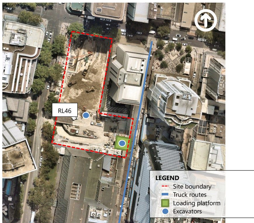
Figure 2.1 – Spoil loading location at VXS worksite
